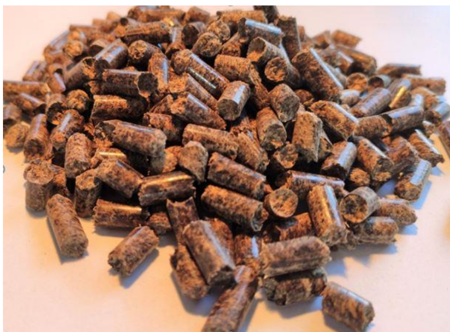
Figure 5: Wood pellets from black thorn ( Acacia mellifera ), IfaS / Amandus Kahl 2020 [calorific value around 5 kWh / kg]
