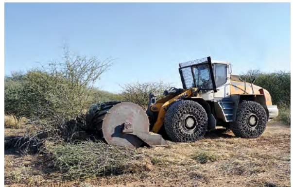
A heavy industrial roller pushed ahead of the tractor is highly efficient and relatively selective.
