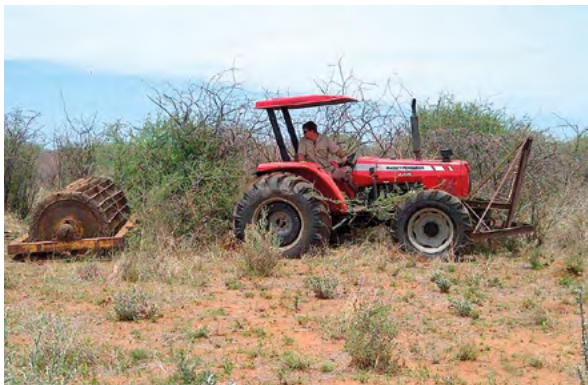
An early, largely home-built roller that proved too light to break large encroacher bush but is effective against smaller bush. The fact that the roller is pulled behind the tractor is a mechanical disadvantage.
