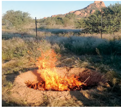
If no kiln is at hand, biochar can also be produced in a hole in the ground.
