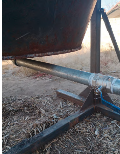
Inlet for quenching from the bottom
