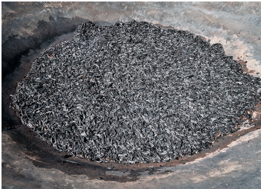
Quenched biochar in a Kon-Tiki kiln after the quench water has been drained off from the bottom.
