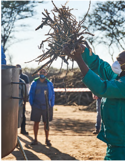
Wood is added from the top of the kiln.
