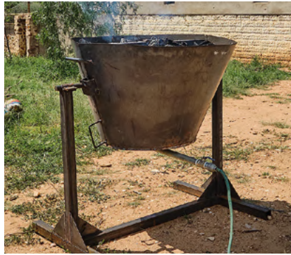
Kon-Tiki kiln with an inlet for direct water supply and swivel technology for easier handling.
