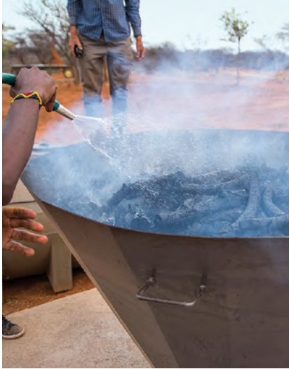
Quenching of biochar with a hose in a Kon-Tiki kiln
